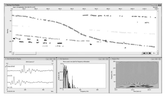
Fig. 3. PAMGuard click detector display showing bearing vs time for 20min of data as the hydrophone array is towed past 8 vocalising whales. All non-sperm whale clicks have been removed from the display. The click waveform, spectrum and Wigner plot are shown for one click (circled) in the centre of the display.
