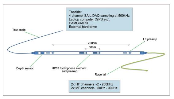
Fig. 2. The Towed PAM system deployed during ObSERVE Acoustic surveys.
