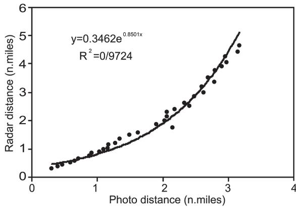
Fig. 5. Relationship between distance measurements to an inflatable small boat target measured by the photographic distance measurement (after Buckland *et al.*, 1993; Gordon, 1990) and by radar during the distance calibration experiment.
