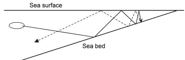
Fig. 6. Schematic of sonar termination in a wedge. An acoustic signal propagating shorewards can turn seawards before it reaches shallow depths, and experiences enhanced attenuation through multiple reflections from the sea surface and the seabed.
