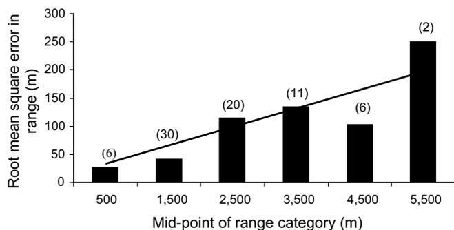
Fig. 5. Mean RMS error in distance estimates to 'growlers' for different distance categories (numbers in brackets indicate sample sizes). Hand held frame, 18m eye height.
