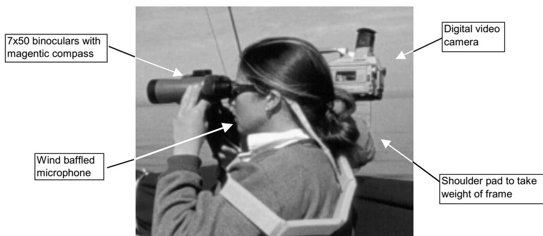
Fig. 3. Use of rigid frame to hold video camera and  $7 \times 50$  binoculars. A downward pointing digital still camera (not shown here) was also attached below the binoculars for taking bearings relative to reference points on deck.
