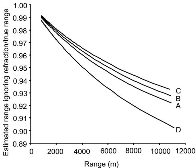
Fig. 2. Ratio of estimated distance ignoring refraction to true distance for three atmospheric profiles. A = Air temp. 0°C, Surface pressure 1,000mB, Temperature gradient  $-6.5^\circ\text{C/km}$ . B = Air temp. 10°C, Surface pressure 1,000mB, Temperature gradient  $-6.5^\circ\text{C/km}$ . C = Air temp. 20°C, Surface pressure 1,000mB, Temperature gradient  $-6.5^\circ\text{C/km}$ . D = Air temp. 0°C, Surface pressure 1,000mB, Temperature gradient  $0^\circ\text{C/km}$ .
