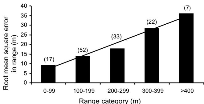
Fig. 6. Combined RMS error for different distance categories from calibration experiments. Hand-held frame. Data from *Song of the Whale* with an eye height of 4m. Numbers in brackets indicate sample sizes.
