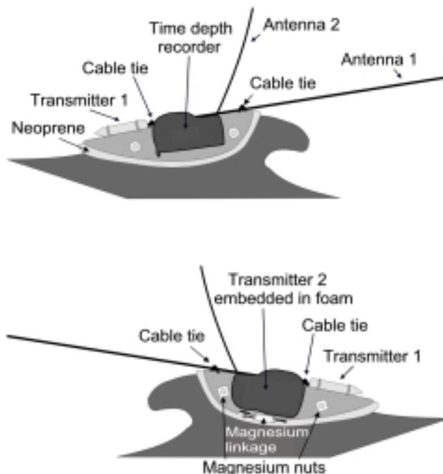
Fig. 1. Diagram of the radiotelemetry package. The *Telonics* transmitter (XTR1) was mounted along the leading edge with the antenna extending aft. A bouyant sub-package consisted of a time-depth recorder (TDR) on the left side of the package and a small ATS transmitter (XTR2) with a near-vertical antenna on the right side.
